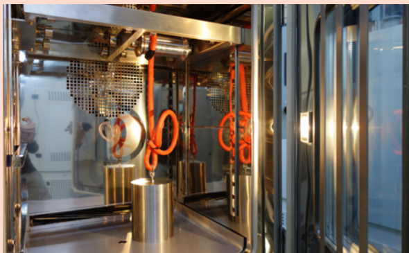
Cold Bend Cables Testing
