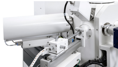
Sense BSD detector for fast TEM like imaging is now available on all GeminiSEMs and Sigmas.
