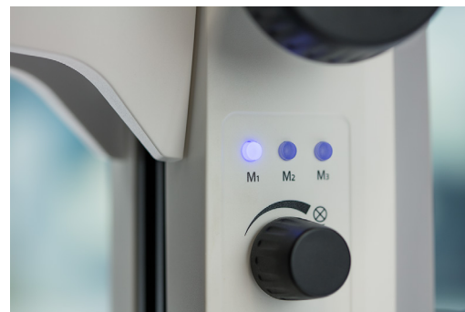
The memory section of stand M LED allows storing and quick recall of up to three customer specific illumination conditions. Press an "M" key long to store, press it short to recall your individual light szenario.
